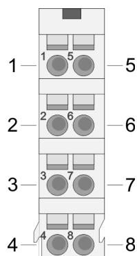
For wires with a cross section of 0.08mm<sup>2</sup> up to 1.5mm<sup>2</sup>.
