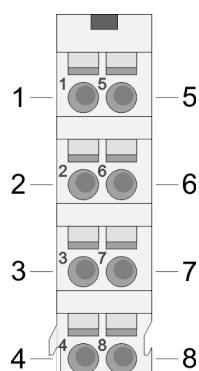
For wires with a cross section of 0.08mm<sup>2</sup> up to 1.5mm<sup>2</sup>.
