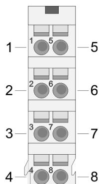
For wires with a cross section of 0.08mm<sup>2</sup> up to 1.5mm<sup>2</sup>.
