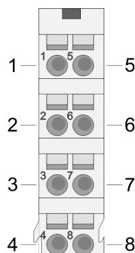
For wires with a cross section of 0.08mm<sup>2</sup> up to 1.5mm<sup>2</sup>.
