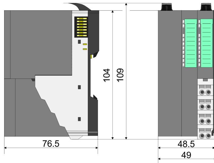
**Dimensions periphery module**
