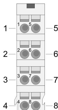
For wires with a cross section of 0.08mm<sup>2</sup> up to 1.5mm<sup>2</sup>.
