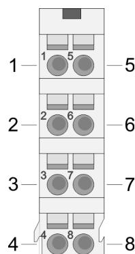
For wires with a cross section of 0.08mm<sup>2</sup> up to 1.5mm<sup>2</sup>.
