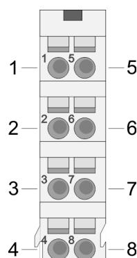
For wires with a cross section of 0.08mm<sup>2</sup> up to 1.5mm<sup>2</sup>.
