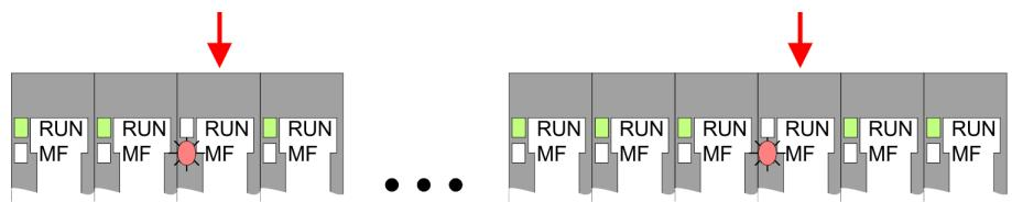
*Behaviour:* After PowerON the MF LED of one module respectively more modules flashes. The RUN LED remains off.
