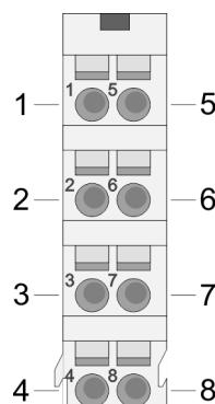
For wires with a cross section of 0.08mm<sup>2</sup> up to 1.5mm<sup>2</sup>.
