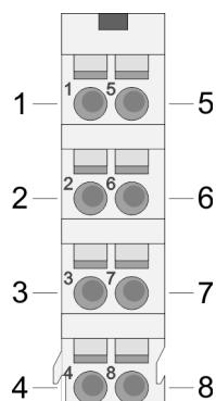
For wires with a cross section of 0.08mm<sup>2</sup> up to 1.5mm<sup>2</sup>.
