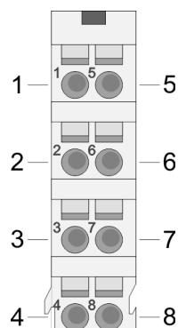
For wires with a cross section of 0.08mm<sup>2</sup> up to 1.5mm<sup>2</sup>.
