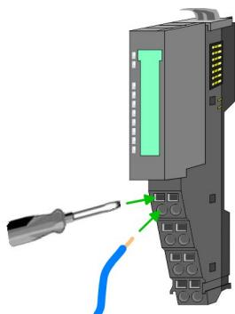
1. Insert a suited screwdriver at an angel into the square opening as shown. Press and hold the screwdriver in the opposite direction to open the contact spring.
