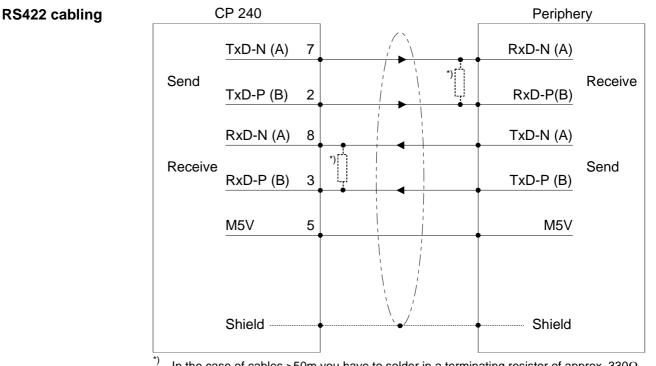
In the case of cables >50m you have to solder in a terminating resistor of approx.  $330\Omega$  on the receiver for data free traffic.
