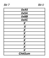
**ERR\_SYNTAX** This telegram is sent automatically through the serial port after the TCM has detected a syntax error in a TCT telegram. Errors can occur in the H\_SEQ, LENGTH, ORG or CHKSUM fields/bytes.
