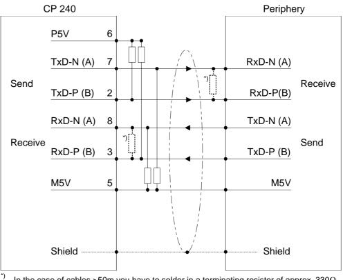
In the case of cables >50m you have to solder in a terminating resistor of approx.  $330\Omega$  on the receiver for data free traffic.
