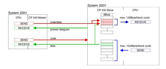
Access to multiple At deployment of multiple slaves with RS485 there cannot occur bus conflict errors because the master may only communicate with one slave at a time. The master sends a command telegram to the save specified via the address and waits for a certain time where within the slave may send its respond telegram. During the latency communication with another slave is not possible.
