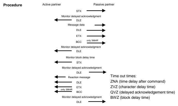
Timeout timesThe QVZ is monitored between STX and DLE and between BCC and DLE.ZVZ is monitored for the entire period of receiving the message.
