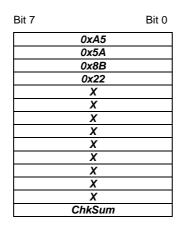
**ERR\_IDRANGE** This message is generated when the user tries to change the ID range base using the SET\_IDBASE command to a value outside the allowed range from 0xFF800000 to 0xFFFFFFF.
