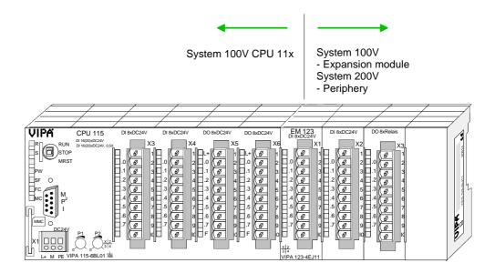
Repeat this procedure with further expansion modules by connecting them via a bus coupler to the right side.
