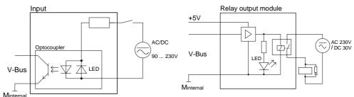
**Note:** When using inductive load please take an suitable protector (i.e. RC combination).
