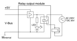
**Note:** When using inductive load please take an suitable protector (i.e. RC combination).
