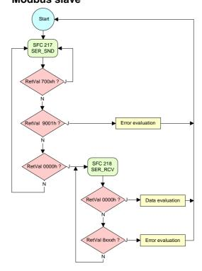
SFC 218 (SER\_RCV) This block receives data via the serial interface.
