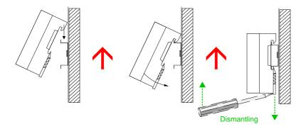
For *mounting*, you set the module onto the head rail from above, using an angle of 45°. Rotate the module down until it clips to the rail with a hearable click.
