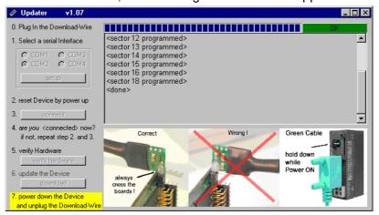
to 7. Turn off the power supply of your CPU, disconnect the Green Cable and turn on the power supply again. Now the CPU is ready with the new firmware.
