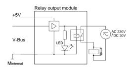
Note: When using inductive load please take a suitable protector (i.e. RC-combination).
