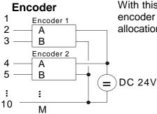
With this functionality 2 encoders can be connected. Configuring "Counter: encoder ..." 2 inputs (A, B) are switched to connect 1 encoder. Here the allocations for the respective 2<sup>nd</sup> input (B) are ignored.
