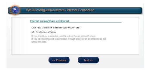
Important for the connection to Talk2M is only a successful Internet connection. Error messages during the test of the online IP address are not relevant.
