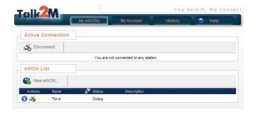
• To establish a VPN connection to your TM click to the connect symbol of the corresponding TM. As soon as the connection is established this is shown at Status with "Connected ...". Now you have direct access to the PLCs connected to the TM.
