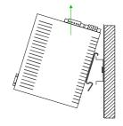
• Now withdraw the module with a slight rotation to the top.
