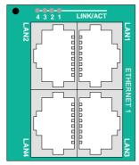
You may connect your TM via Ethernet to the local machine network. Via Ethernet the integrated Web page of the TM module may be accessed for according configurations.
