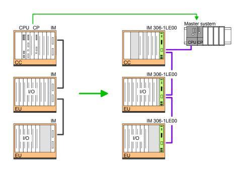
Deployment IM 306-1LZ00 IM 306-1LE00 (interrupt capability) If you want the support of modules with interrupt capability, this structure is to be used:
