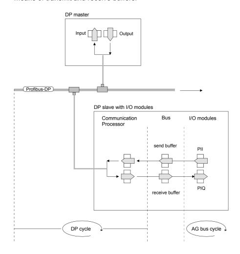
PII: process image of the inputs PIQ: process image of the outputs Function Acyclic data communication (DP-V1) The key feature of version DP-V1 is the extended function for acyclic data communication. This forms the requirement for parameterization and calibration of the field devices over the bus during runtime and for the introduction of confirmed alarm messages.
