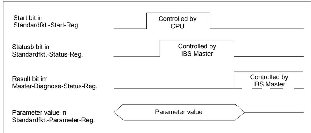
The diagram in the picture above shows the handshake mechanism at usage of the standard functions. A "0" in Bit 10 (RESULT) of the master diagnosis status register shows that the standard function has been finished successful.
