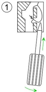
You may connect wires with a cross-section of 0.08mm<sup>2</sup> to 2.5mm<sup>2</sup>. You can use flexible wires without end case as well as stiff wires.
