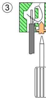
Here also you may connect wires with a cross-section of  $0.08\text{mm}^2$  to  $2.5\text{mm}^2$ . You can use flexible wires without end case as well as stiff wires.
