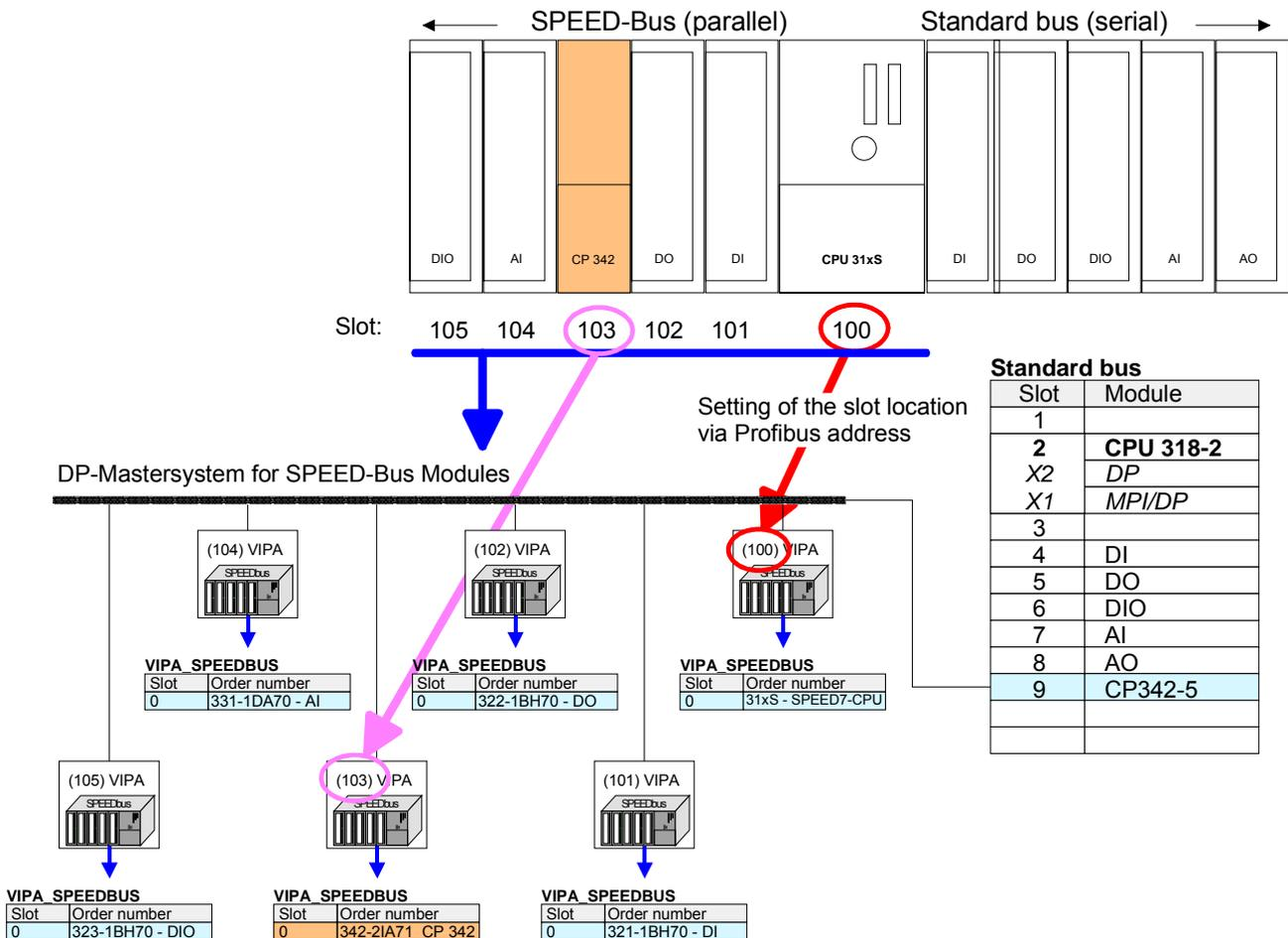
The according module is to be taken over from the HW Catalog of VIPA\_SPEEDBUS to slot 0.
