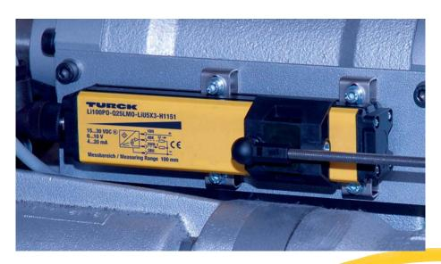
The new inductive linear position sensor by TURCK operates on the basis of a completely new, revolutionary measuring principle. The positive features of standard measuring systems are combined and systematically developed further. The position is not detected via a positioning magnet but via an inductive oscillating circuit. The sensor is thus completely immune to magnetic fields which are generated by large motors for example.
