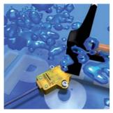
Made of high-quality plastic and IP67 rated, the housing provides high mechanical stability, protecting the sensor optimally against most chemicals and oils. The two-part build consisting of sensor and positioning element compensates lateral offsets of ≤ 3 mm and guarantees easy fitting and operation.
