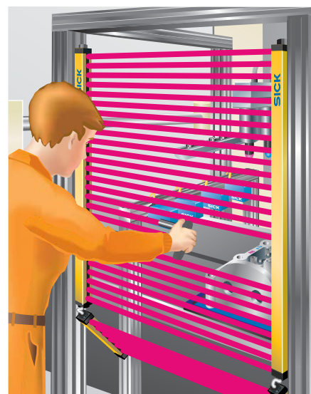
C 2000 cascadable on a pad printing machine
