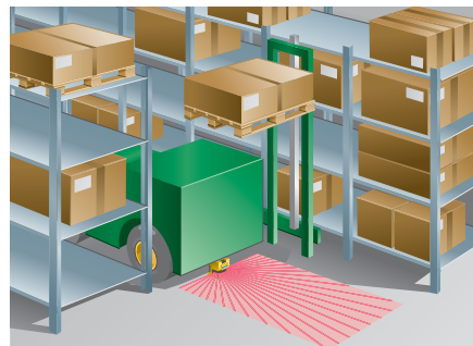
Hazardous area protection on a narrow aisle stacker
