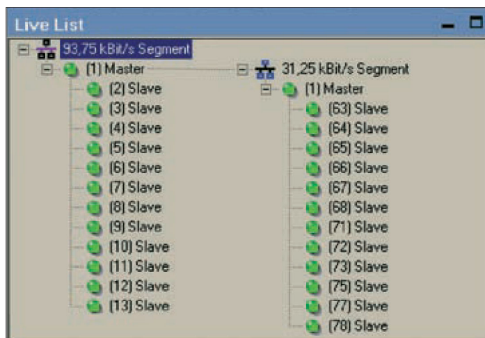
Fig. 4 - Live-List (DP- / PA-Communication)
