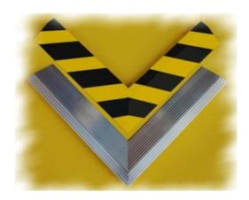
The **AM Safety** frame profile AF is mounted on the edges of the walkable sides of the safety mat. Due to the bevel of the profile the risk of stumbling is successfully prevented. The frame profile is produced as specified, mitred and step-drilled.
