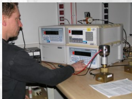
Mounting, final check with calibration-report
